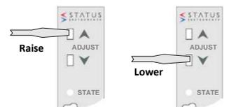
4.0 Once adjust is complete allow 30 seconds with no button press, the conditioner will time out and return to normal operation.
