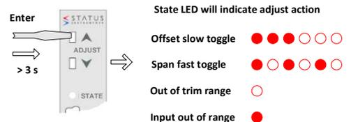
3.0 Adjust output voltage by pressing either the raise or lower button, single click to step advance, or press continuously to auto advance.
