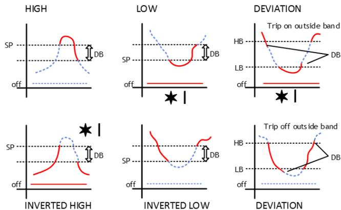
\*1 **Latching** type relays are used; on loss of input signal/power, a set-low alarm will be recognised and held.
