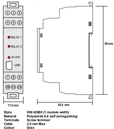
The equipment must be mounted on a DIN rail style DIN EN50022 inside a plastic or metal enclosure with a protection level >= IP65. All wiring must be secured. Maximum cable sizes 2.5 mm<sup>2</sup>. Connection is via screw clamp terminals.
